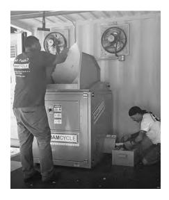
LRPC is working with Gilford DPW to acquire grant funding to pay for the remaining balance of the Gilford densifier unit patented by Foam Cycle LLC. This unit is key to preparing foam for processing and transport to a vendor who can reuse the densified foam (ingots) to make new products such as insulation, molding,
